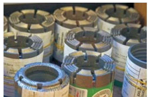
Figure 4. Diamond-impregnated drilling bits enable the ANDRILL drilling system to recover high-quality core, with up to 98% core recovery through glacial and glaci-marine sediments.
